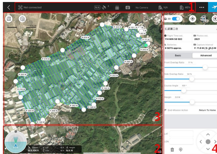
Figure 1. UAV flight path generated using DJI GS Pro software to ensure optimal site coverage and image overlap.
